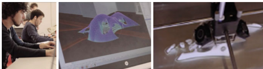
Fig. 12.7 NC design to additive production of porous structures implemented at Hyperbody, TUD (2014)
